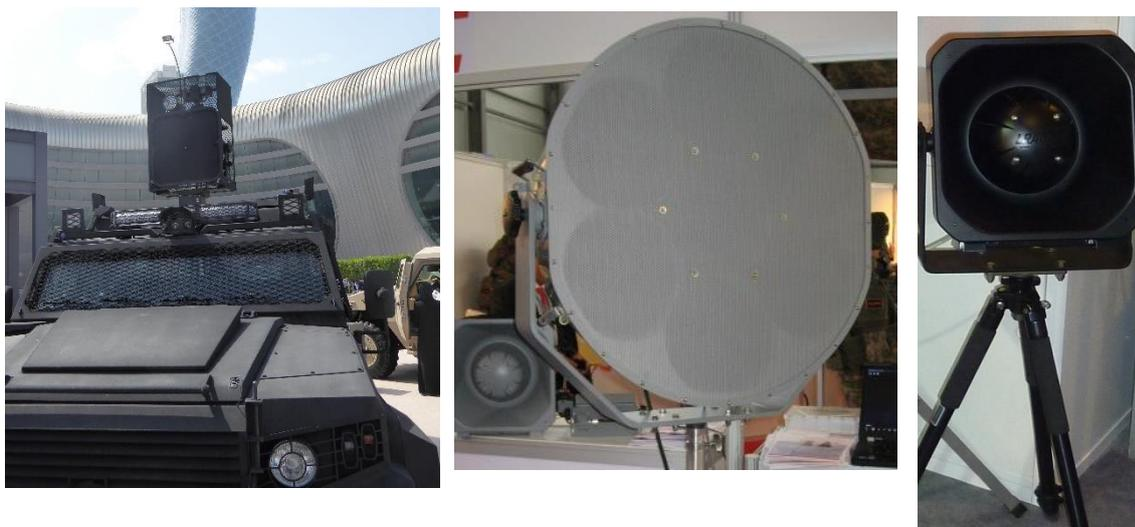
*Left: Vehicle-mounted; Centre: Free-standing; Right: Free-standing acoustic devices. ©Robin Ballantyne, Omega Research Foundation.*
